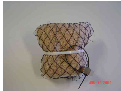
Plate 1. A. Multiplate samplers constructed from hardboard (left) and perspex (right) showing position of samplers in relation to the concrete paver. Arrow indicates attachment point for the coir sampler. B. Coir sampler viewed from bottom showing the weight on a plastic tie, the black coarse mesh enveloping the folded coir mat, and the 0.5 mm mesh which covers the lower half of the coir sampler to prevent loss of macroinvertebrates during removal.
