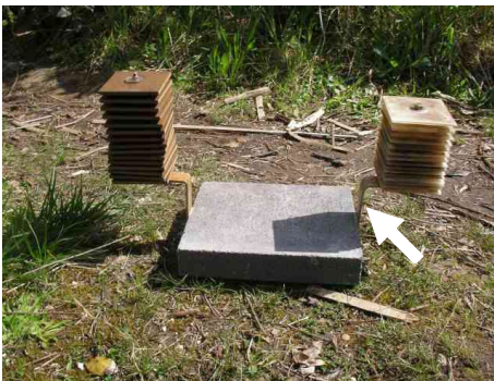
Plate 1. A. Multiplate samplers constructed from hardboard (left) and perspex (right) showing position of samplers in relation to the concrete paver. Arrow indicates attachment point for the coir sampler. B. Coir sampler viewed from bottom showing the weight on a plastic tie, the black coarse mesh enveloping the folded coir mat, and the 0.5 mm mesh which covers the lower half of the coir sampler to prevent loss of macroinvertebrates during removal.
